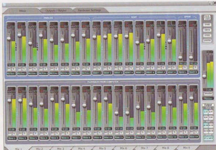
The FireStudio's Control Console software, with the Mixer page open.
